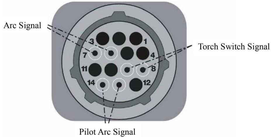
Refer to the following table when connecting the ADVANCECUT system to a torch height controller or CNC controller with a machine interface cable.
